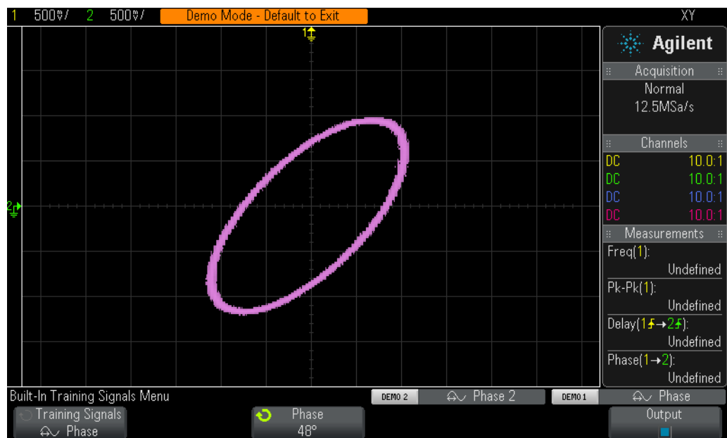
Figure 40 A Lissajous pattern using a scope's XY mode of two sine waves of the same frequency, but 48 degrees out of phase with each other
