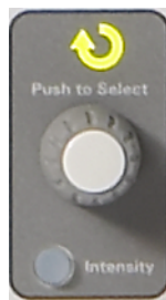
Figure 7 Oscilloscope general-entry control
