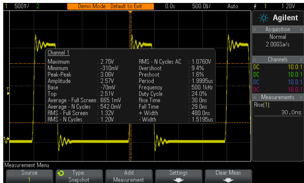
Figure 35 Performing a comprehensive set of automatic parametric measurements using the “Snapshot All” function
