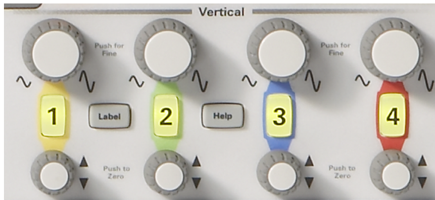
Figure 5 Oscilloscope vertical (Y-axis) controls
