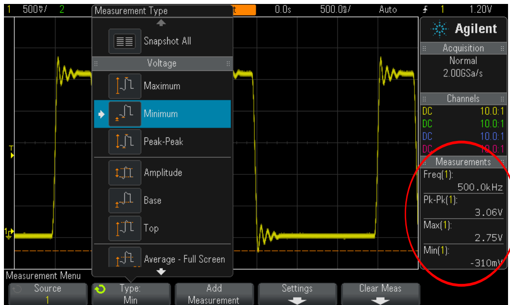
Figure 32 The scope automatically performs up to four parametric measurements
