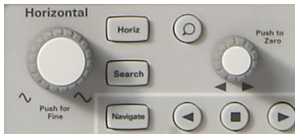
Figure 4 Oscilloscope horizontal (X-axis) controls
